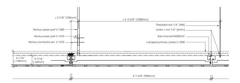
MAGNETIC SYSTEM WITH CLOSED BACKING
