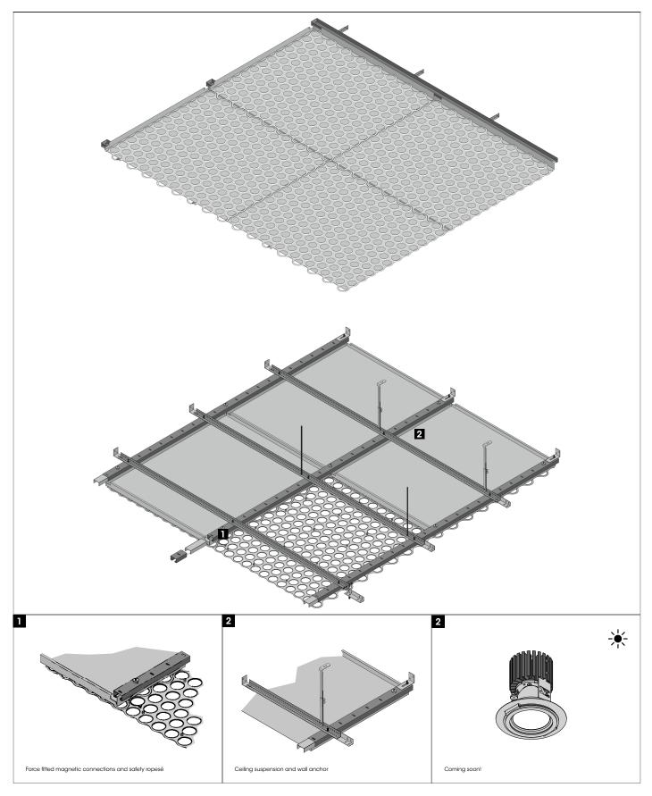
MAGNETIC SYSTEM WITH CLOSED BACKING
