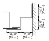
F 2025 shadow gap wall angle For perimeter panels, to be cut on site
