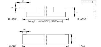
AS 30: H= 1 3/16" [30mm] | z= 9/16" [14mm] | x= 3/16" [5mm] AL 2: H= 1 9/16"[40mm] | w= 15/32" [12mm]
