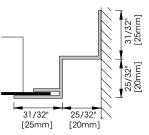
F 2025 shadow gap wall angle For perimeter panels, to be cut on site
