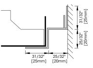
F 2025 shadow gap wall angle For lay-on perimeter panels
