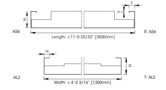
AS 6: H= 1 3/16" [30mm] | z= 13/32" [10mm] | x= 3/16" [5mm] AL 2: H= 1 3/16"-2 3/8" [30-60mm] | w= 15/32" [12mm]
